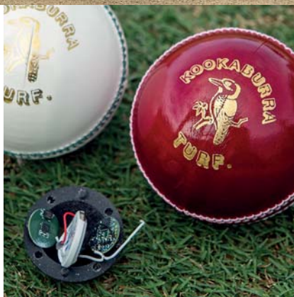
Sportcor's Smart Ball can measure spin and speed
